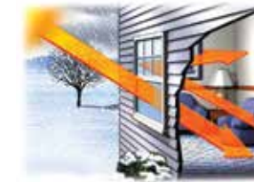
In winter months, Low-E glass lets warm solar rays into your home, while preventing indoor heat from escaping.
